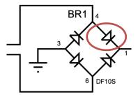
With the In Circuit test, it is possible to verify the presence, the correct mounting and the electrical characteristics of the diodes that will be mounted, ensuring the reliability of the product over time.
